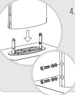
4. Slide the Solar Pillar (Part A) over the Mounting Bracket (Part B) and secure using the four screws (removed from the Pillar earlier) and the Allen Wrench (Part E).
