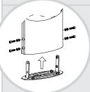
2. Remove the Mounting Bracket (**Part B**) from the Solar Pillar (**Part A**) by removing the four screws and sliding the bracket away from the bottom.
